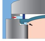
Door closed, circumferential locking ring in locking position. The internal steam pressure presses the lip seal between door and chamber.
