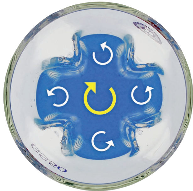
GS vessel principle (viewed from above)
