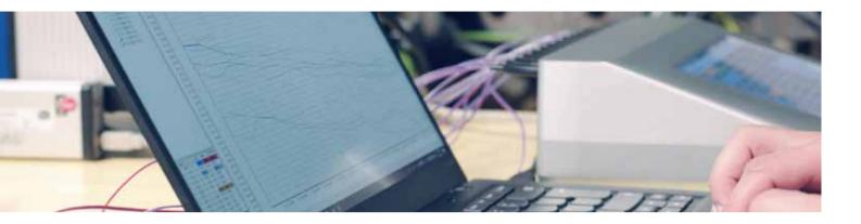
The E-Val Pro Thermal Validation System is designed for validation applications that require compliance with FDA guidelines and international GMP standards. The E-Val Pro greatly simplifies and correctly documents the entire validation process. The ValSuite Pro software keeps a complete database on all aspects of your validation requirements - tracking thermocouples, calibration reports, test setup, data analysis, specific user access and final compliance reports.
