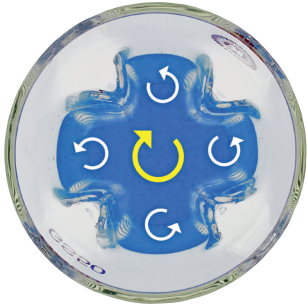
GS vessel principle (viewed from top)
