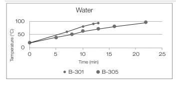
$\Delta T_{70~^{\circ}\text{C (water)}}$  : B-301 -> 13 min; B-305 -> 22 min
